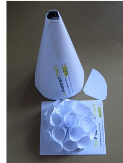
the assembly of the CSFE from printed template then filled with sand contained in a plastic sleeve / liner.
